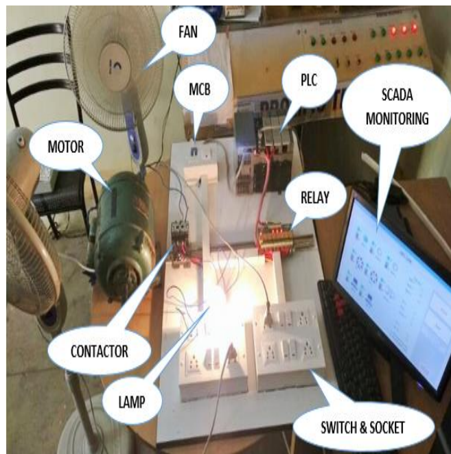
Fig 8: Controlling and monitoring the hardware kit through SCADA system.
